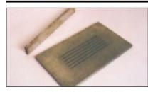
MPI TEST BAR/MPI TEST BLOCK Contains artificial discontinuities for Magnetic particle Inspection.
