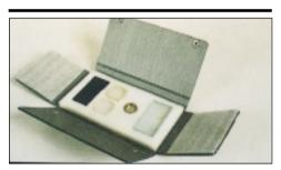
SPOT MENISCUS KIT. PART NO. 240045 Used to check the sensitivity of the penetrant. The penetrant when sandwiched between lens and a plain glass will show a white spot. Smaller the white spot, better the sensitivity.
