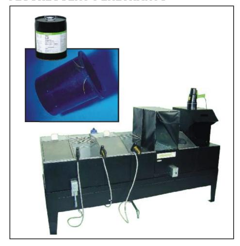
Zyglo® Fluorescent Penetrant Testing is the most versatile and reliable process for the detection of defects open to the surface in non-porous materials, both metallic and non-metallic.
